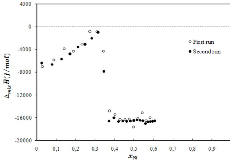
**Figure 2:** Partial molar enthalpies of mixing at 1273 K in liquid Bi-Ni alloys. Standard states: pure liquid metals.
