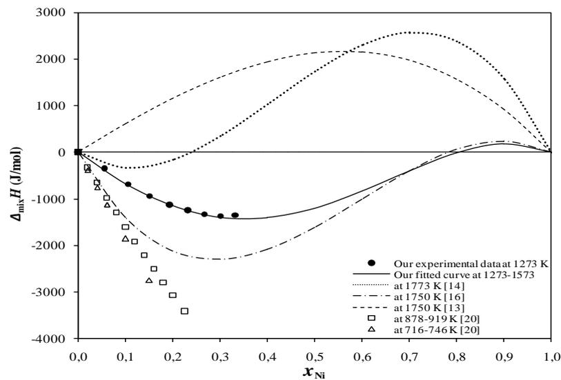
**Figure 4:** Comparison of experimental and calculated enthalpies of mixing values in the liquid Bi-Ni system.
