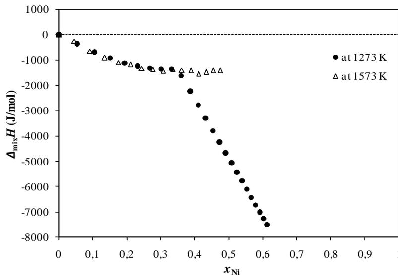
**Figure 3:** Integral molar enthalpies of mixing at 1273 and 1573 K in liquid Bi-Ni alloys. Standard states: pure liquid metals.
